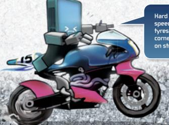
Hard tyres wear well and allow high speeds, but they don't grip well. Soft tyres give good grip when braking and cornering, but they slow the bike down on straight sections.
